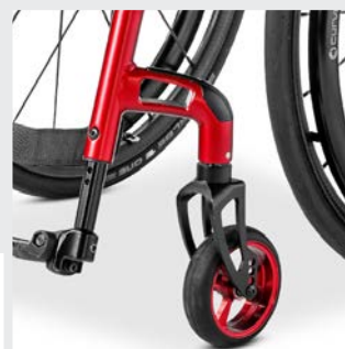
Castor wheel connection milled from solid material
