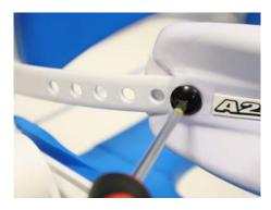
• To adjust the depth of the belt, loosen the screw connection as shown and select the desired position.
