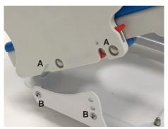
A = Guide slots of the seat unit B = Locking shafts of the base
