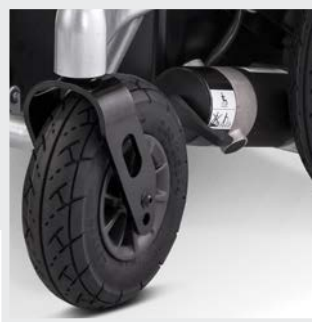
Castor wheels with aluminium rim
