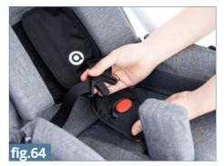
There is a possibility of adjusting the length of the 5-point belts with the use of the buckle showed in the photographs (fig. 65, 66).
