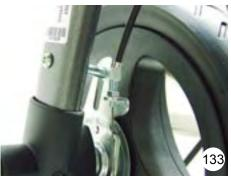
After loosening the counternut the initial tension can be adjusted by screwing the guide of the bowden cable.
