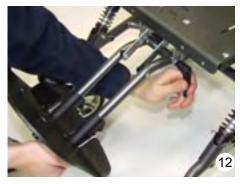
If your **BINGO Evolution** is equipped with an angle adjustable footrest hanger the footrest could be in a hinged position for the transport.
