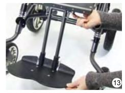
If your **BINGO Evolution** is equipped with a footrest hanger 90° the footrest could be in a hinged position for the transport.
