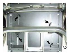
After loosening the wing nuts under the seat it is possible to adjust the seat width continuously variable by sliding the hip supports respectively the thigh supports.
