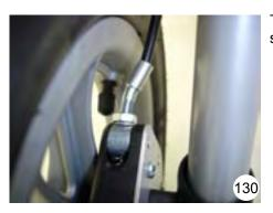
Tighten the counter nut firmly again and ensure that the crank of the set screw shows towards the rear frame, away from the tire.
