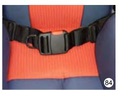
Open the lap belt by pushing the red key on the buckle.
