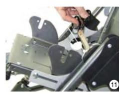
• Cut the transport safety (cable connector) carefully.
