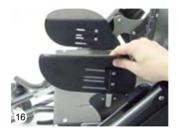
• Pull the hip support upholstery from the top onto the bracket, so that the cushioned side points to the inner side and fix it with the Velcro fasteners.
