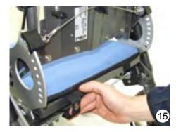
• Fix the snap fasteners below the backmost seat edge also (15).
