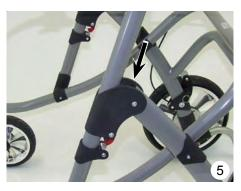
• Push down the sliders (5) until the red safety hooks lock with an audible click.
